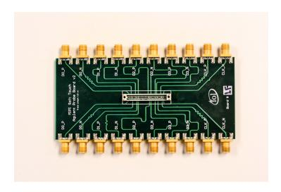
The Soft-Touch board is designed to be used with the Agilent U4421A Protocol Analyzer for MIPI D-PHY Interfaces. The Soft-Touch board can be used to monitor traffic between two MIPI D-PHY devices, or between the U4421A Protocol Exerciser and a MIPI D-PHY device under test.
