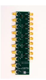
The P331 MIPI D-PHY/CSI/DSI Probing Board is designed to attach directly to a Moving Pixel Company P331 D-PHY Generator using short SMA barrels. It allows convenient connectivity for an Oscilloscope or Logic Analyzer system in order to monitor an active D-PHY based link. There are test points which can be a convenient point for solder-in style probe points.
