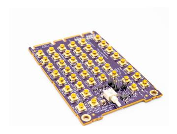
Signal Integrity Board for OCP 3.0 SI Transmitter Gen 4 (16GT/s) used for testing Root Complex Transmitters and Receiver Calibration (paired with the CBB) of AIC Receivers. Additionally these fixtures can be used in the same fashion for validating PCIe SSDs using the EDSFF form factor for E1.L, E1.S, and E3.
