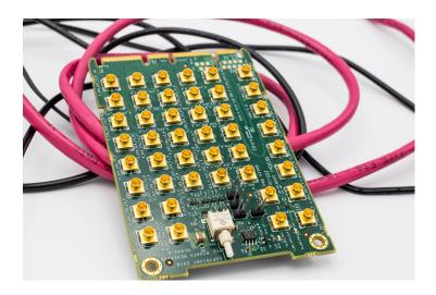
Signal Integrity Board for OCP 3.0 SI Transmitter Gen 3 (8GT/s) used for testing Root Complex Transmitters and Receiver Calibration (paired with the CBB) of AIC Receivers. Additionally these fixtures can be used in the same fashion for validating PCIe SSDs using the EDSFF form factor for E1.L, E1.S, and E3.
