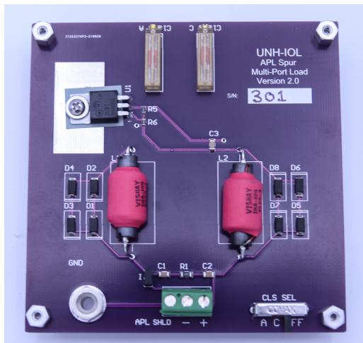
Printed Circuit Board featuring terminal block connection that provides an active Spur Load for power classes A, C. This board is used in multiples to load additional ports of a Spur Power field switch with more than one port for System.1.1 tests in the Annex of the APL Power Conformance Test Specification.
