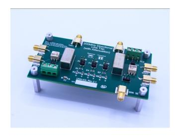
Printed Circuit Board featuring a terminal block connection, directional couplers and SMA Connections for real-time capturing of link signalling on test and measurement equipment. This Line-tap Board is useful for Group 3 and 4 of Section 146 as well as all of Section 98 as defined in the APL Data CTS.
